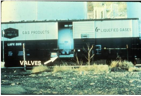
Older style cryogenic tank inside of a box car.
