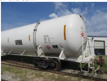
They have a pressure relief system to "self vent" the product when the pressure gets high on the outside of the car.
