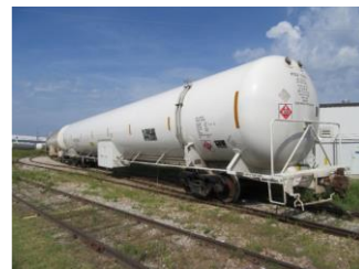
These tank cars have an inner tank and an outer tank. There is a "vacuum" in the space between them to help keep the product cold.
