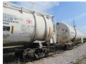
Load/Unload boxes are on ends or sides
