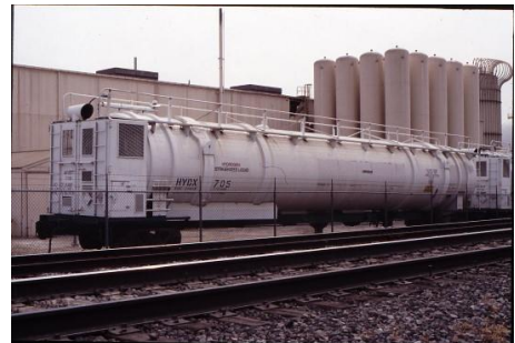
Older style cryogenic tank car transporting liquid hydrogen.
