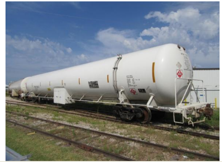
Liquid Natural Gas is a future product for these cryogenic tank cars to transport.
